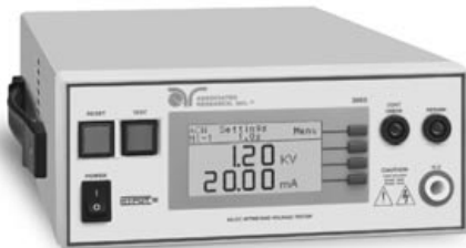
(Figure 5) Hypot®III Model 3665 with manual reset and audible and visual failure indicators.
